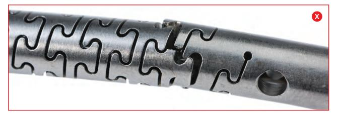
• Cracked/Fractured in flexible shaft body
