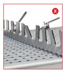
Bent, bowed or warped:
