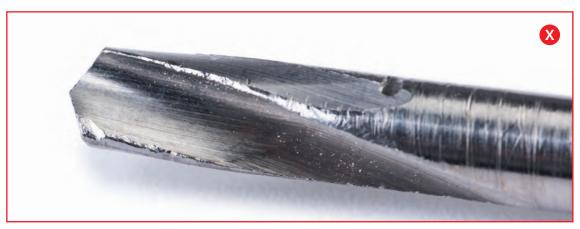
• Damaged cutting edges
