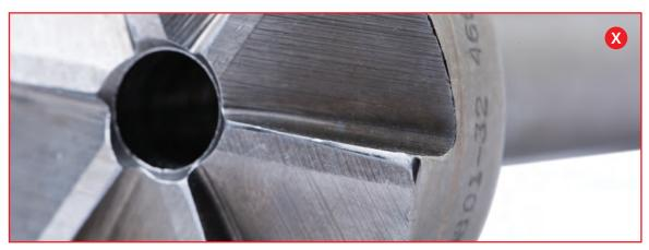
• Damaged cutting edges
