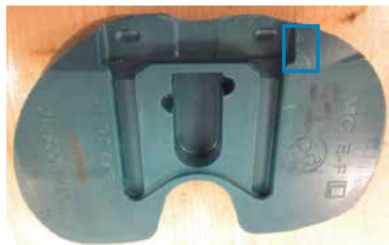
TASP TOPS Cracks along length of dovetail
