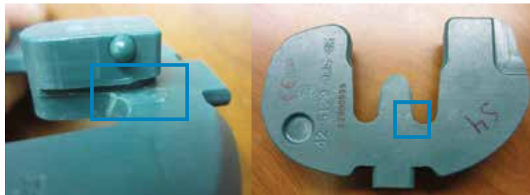
TASP BOTTOM Cracks/crazing along central post
