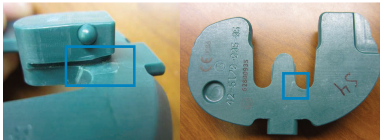
TASP BOTTOM Cracks/crazing along central post
