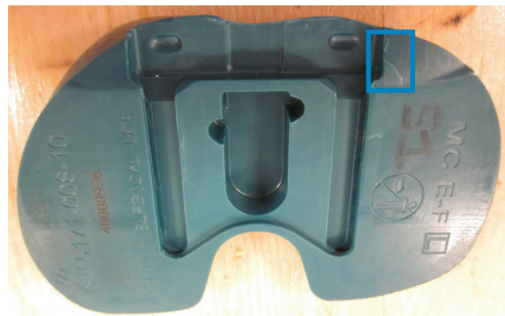
TASP TOPS Cracks along length of dovetail
