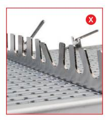
Bent, bowed or warped:
