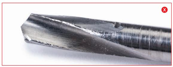
• Damaged cutting edges
