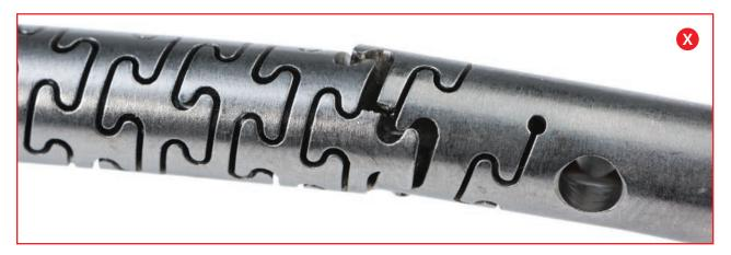
• Cracked/Fractured in flexible shaft body
