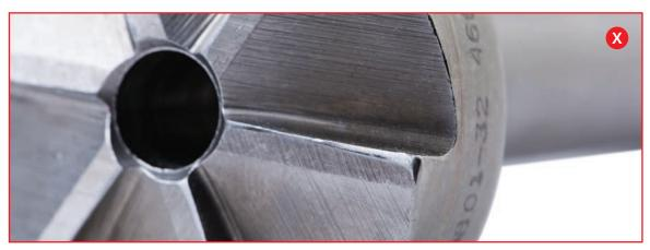
• Damaged cutting edges
