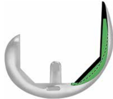
Figure 4 Standard Trochlear Groove (Green) vs. Vanguard Deeper/ Swept-back Trochlear Groove
