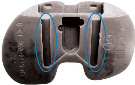
Deformation along edges of dovetail
