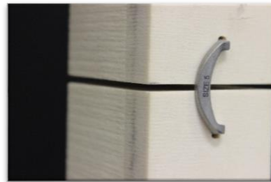
FIGURE 2: THE STAPLE IMPLANTED ACROSS THE FRACTURE SITE
