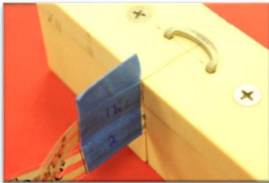
FIGURE 5: CLOSER VIEW OF THE TWO FLEXIFORCE SENSORS (1-PROXIMAL, 2-DISTAL) WITHIN THE CONSTRUCT
