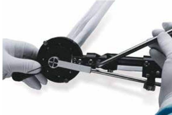
Adjustment of central component to allow target wire to pass through center of target disc
