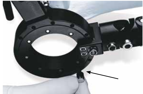
Application of range of motion limit pins
