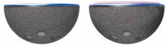
Correct Ceramic Liner Seating
