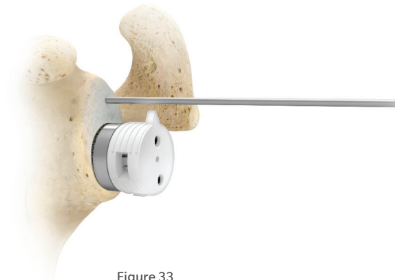
Figure 33 Insert the Signature™ ONE Screw Guide into the cavity of the base plate. Ensure guide protrusions mate with screw holes on the base plate and guide arrow is positioned superiorly.
