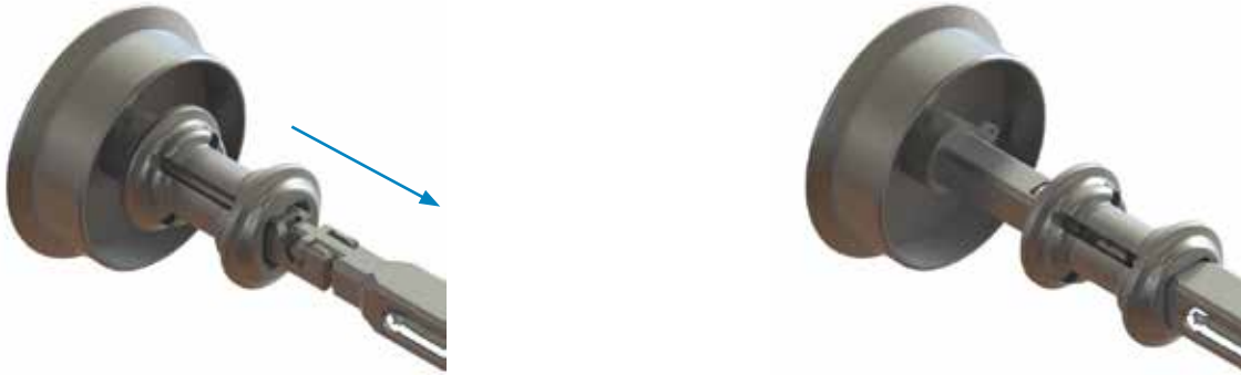
Figure 16: ROSA Quick Connect Sleeve sliding along the interface to lock the installation
