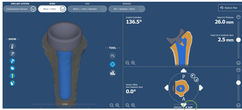
Figure 14 - Stem is selected, allowing the user to show the manipulator in transverse view and move the implant
