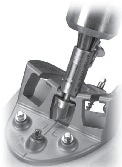
Fig. 10 Place PFJ Drill Milling Adapter into track before initiating power
