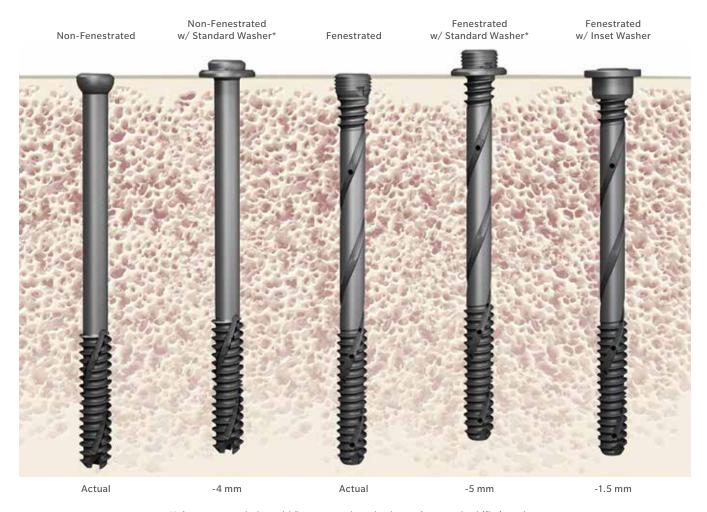
$^{\star}\text{It}$  is recommended to add 5 mm screw length when using standard (flat) washer.
